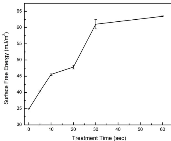
Fig. 3. Surface free energy ( $\gamma$ ) of PET surface as a function of treatment time for 50 Hz DBD at near-atmospheric pressure.
