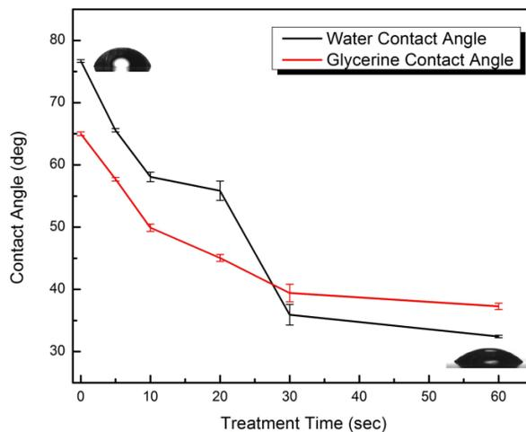
Fig. 2 Contact angle of PET surface as a function of treatment time for 50 Hz DBD at near-atmospheric pressure.
