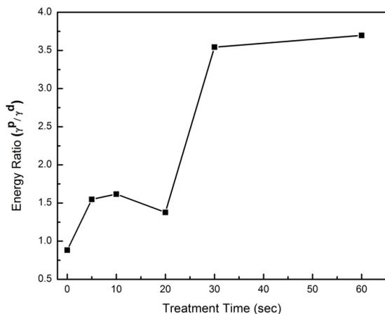
Fig. 4 Energy ratio as a function of treatment time for 50Hz DBD at near-atmospheric
