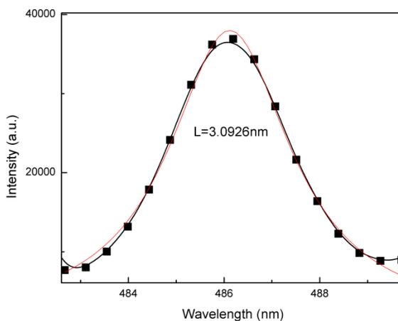
Fig. 5 Recorded line profile for  $\Delta\lambda=3.0926\text{nm}$  and its Lorentzian fit
